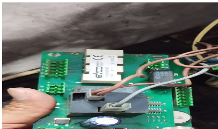
Controller PCB of 4°C Fridge
