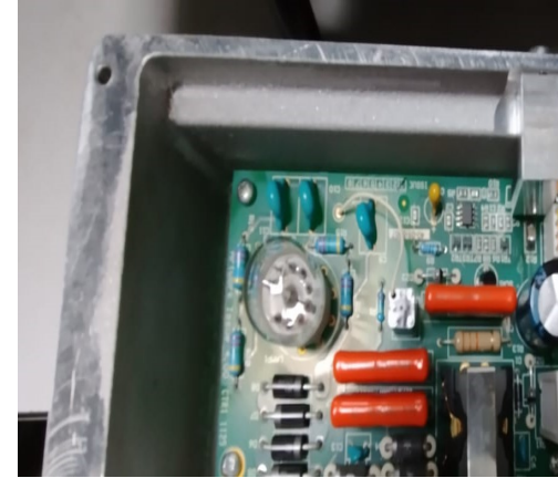
Power Supply of Vacuum Pump
